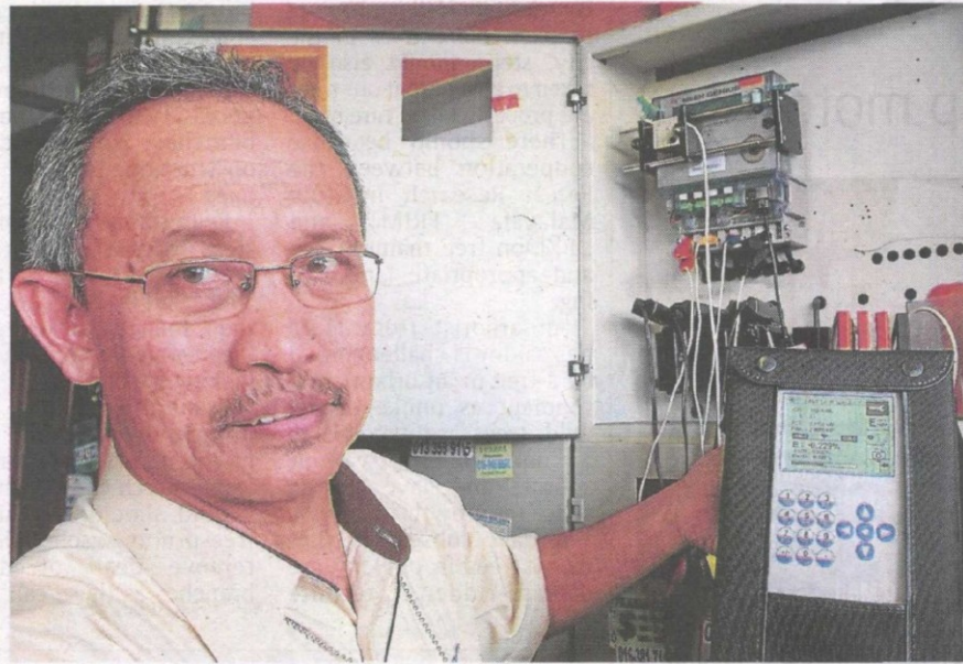
Checking its accuracy: Othman showing how the Portable Test Set for Electricity Meter is used to test the accuracy of consumers' electrical meters during a site inspection of electricity meters at a commercial premises in Taman Kajang Sentral, Kajang.
