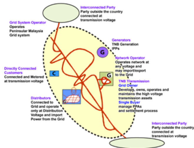
Figure 20: Parties in the Grid Code
